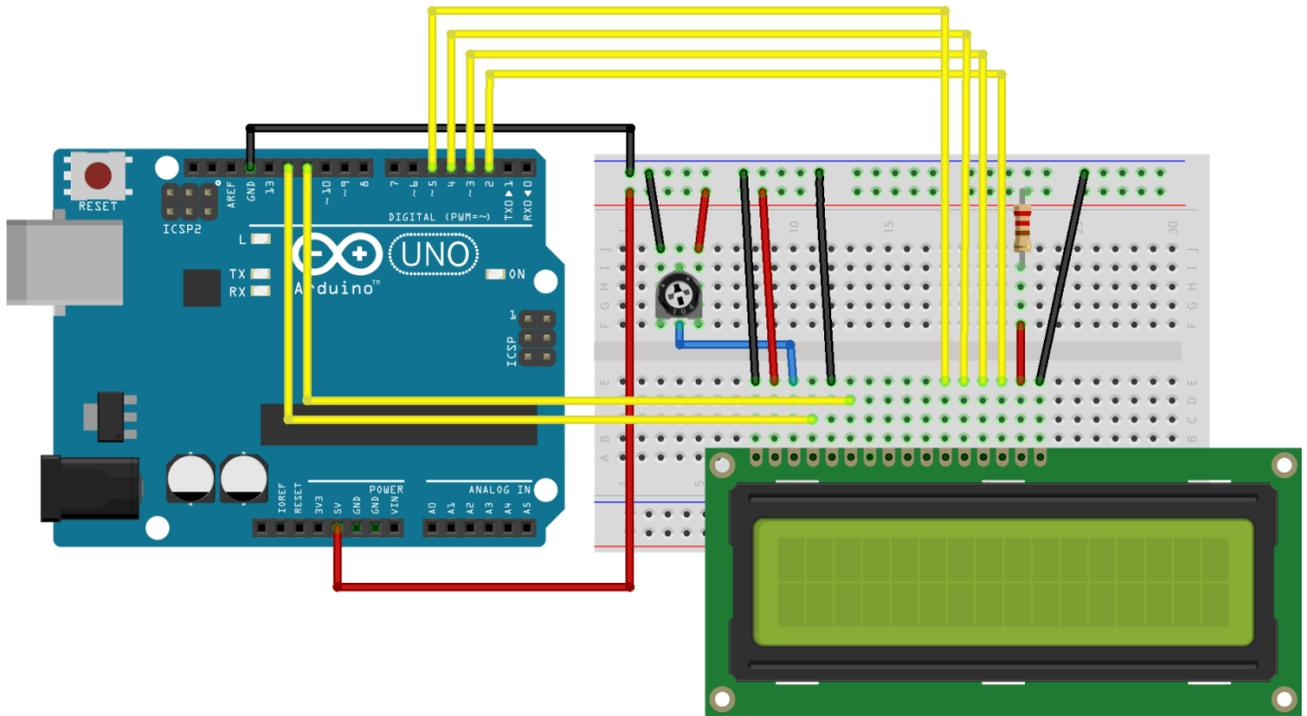
Fig 17 :- Connection of the LCD display with ARDUINO
