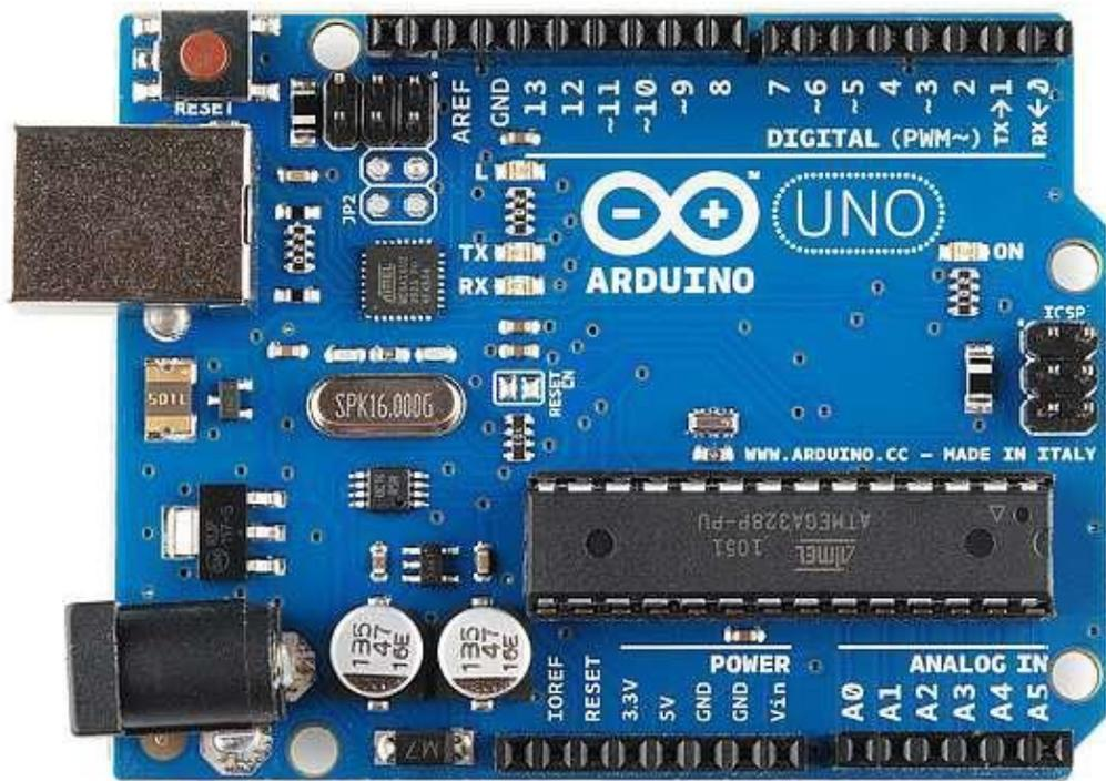
Fig. 4 :- Real Arduino UNO board
