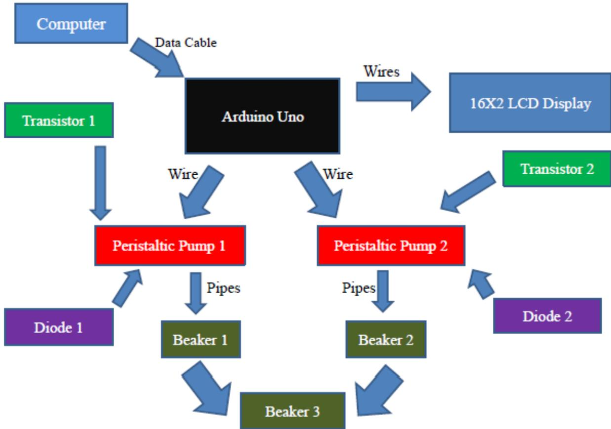
Fig 1:- Block diagram of the proposed project
