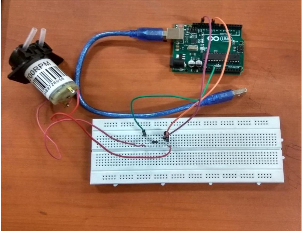
Fig 18 :- Connection of the pump with ARDUINO in a breadboard
