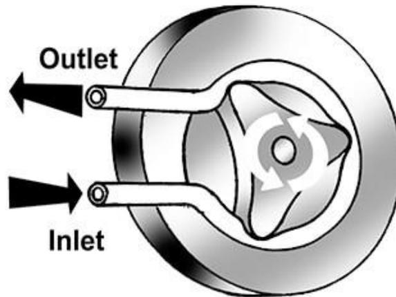
Fig 3:- Mechanism of Peristaltic Pump
