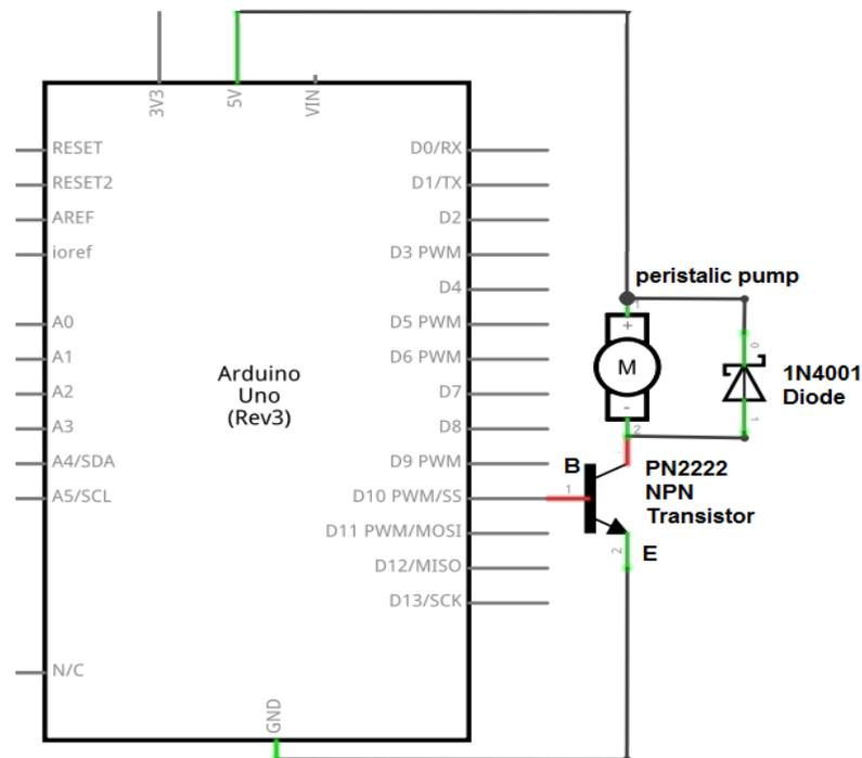
Fig 16 :- Connection of the pump with ARDUINO
