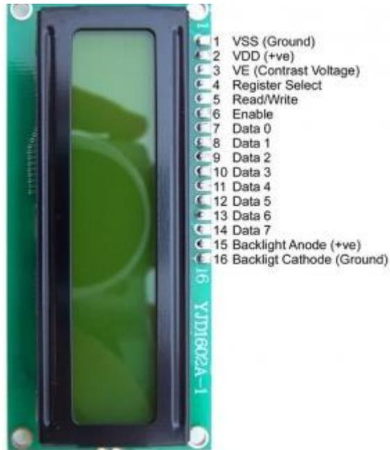
Fig 8 :- A 16x2 LCD display with pin layout
