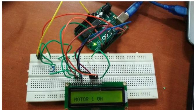
Fig 19 :- Displaying “MOTOR 1 ON” command
